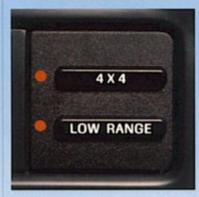
Shift from 2-wheel drive to 4-wheel high and back again" on the fly" with Electric Touch Drive — at the touch of a button.
