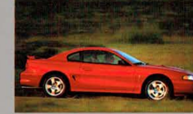
1996-1998 SVT MUSTANG COBRA 305 horsepower 4.6-liter obj V8 T45 five-speed manual transmission 13-in. front discs, PBR calipers; 11.65-in. rears Production: 28,709 units
