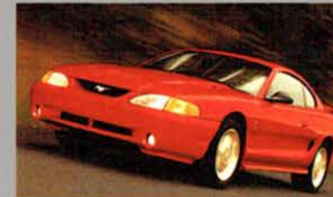
1994-1995 SVT MUSTANG COBRA 240 horsepower 5.0-liter obj V8 T5 five-speed manual transmission 13-in. front discs, PBR calipers; 11.65-in. rears Production: 11,017 units
