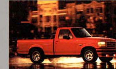
1993-1995 SVT F-150 LIGHTNING 240 horsepower 5.8-liter obj V8 E4OD four-speed automatic transmission Tow rating: 5,000 lbs.; payload: 745 lbs. Production: 11,563 Units
