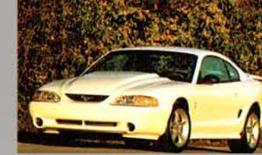
1995 SVT MUSTANG COBRA R 300 horsepower 5.8-liter obj V8 Tremec five-speed manual transmission Lightweight street-legal racing model Production: 250 units
