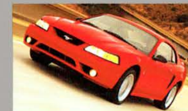
1999 SVT MUSTANG COBRA 320 horsepower 4.6-liter obj V8 Independent rear suspension introduced Traction control introduced Production: 8,000 units (estimate)
