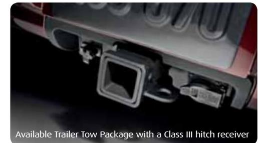
Available Trailer Tow Package with a Class III hitch receiver
