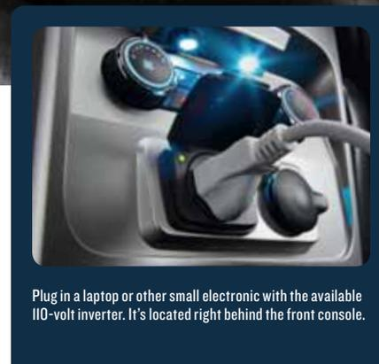
Plug in a laptop or other small electronic with the available 110-volt inverter. It's located right behind the front console.
