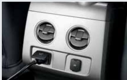
**NEW 110-VOLT POWER INVERTER** is conveniently located on the back of the available flow-through center console.
