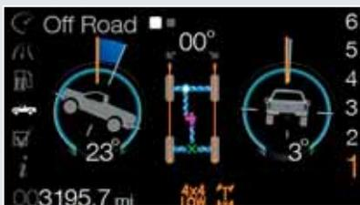
**CLASS-EXCLUSIVE OFF-ROAD DISPLAY** in the available new LCD Productivity Screen gives you instant feedback on pitch angle, wheel direction and bank angle for more precise maneuvering over treacherous terrain.
