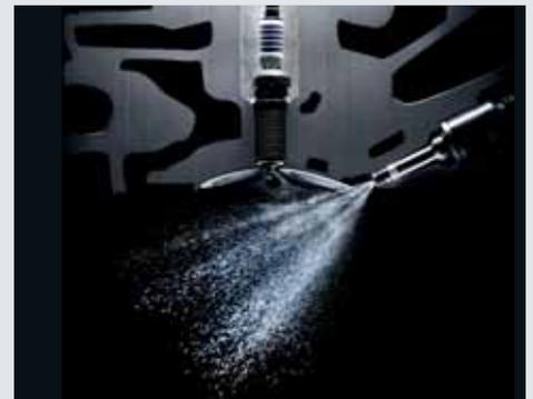
**HIGH-PRESSURE DIRECT INJECTION** employs a precise spray pattern to disperse fuel directly into the chamber during intake, contributing to clean, fuel-efficient operation. Fuel literally atomizes with pressurized air before the spark ignites the mixture during the compression stroke. Combining the proven diesel truck engine technologies of direct injection and turbocharging in this new gasoline engine results in smooth, immediate acceleration. In any gear. At any speed.
