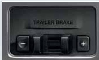
**TRAILER BRAKE CONTROLLER<sup>3</sup>** is a factory-integrated option that uses braking input, vehicle speed and information from the vehicle's Anti-Lock Brake System (ABS) to balance the performance of the truck brakes and electric trailer brakes.
