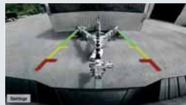
**REAR VIEW CAMERA** option displays a full-color image in your auto-dimming rearview mirror or on the available Navigation System's 8-in. screen (shown). Just shift into Reverse for a wide-angle view behind the truck, complete with a distance guide. The rearview mirror display is 37.5% larger this year.
