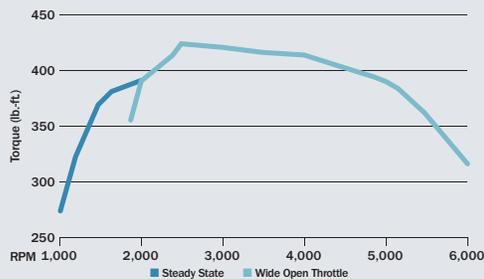
**TORQUE BEATS ALL COMPETITORS** with the new 3.5L EcoBoost Ti-VCT. It reaches over 90% of peak torque way down at 1,700 rpm and holds strong all the way up through 5,000 rpm.
