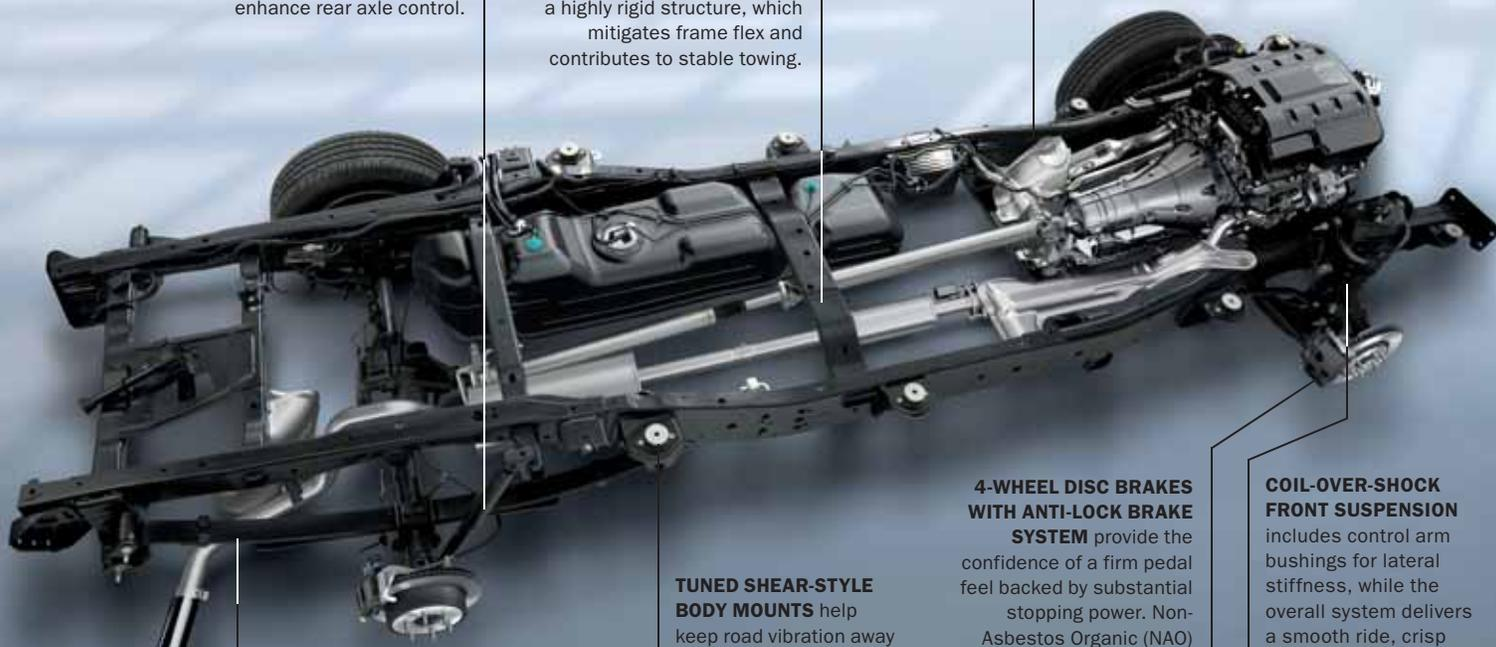
**WIDE REAR LEAF SPRINGS** provide outstanding axle control, while balancing ride smoothness with best-in-class load capability.
