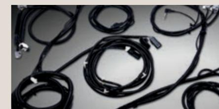
**Wiring harness (Sedan).** Includes (2) light connectors that support up to (3) LED lights each (engine compartment); (1) grille LED light connector that supports (2) LED lights; (2) 50-amp battery ground circuits in power distribution junction block (in-trunk); (1) 10-amp siren/speaker circuit (engine to trunk); trunk circulation fan; trunk electronics tray (4 sq. ft.); and pre-wiring for grille LEDs and siren/speaker.
