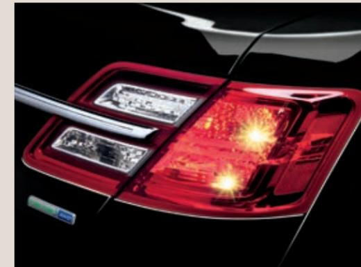
**Police taillamp.** Includes halogen base lamp, plus (2) integrated hemispheric lighthead LED side warning lights.
