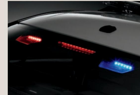
**Police back-window lights.** Includes (2) backlit flashing, linear high-intensity LED lights with surround cover (driver side red; passenger side blue) – mounted inside the back window glass.
