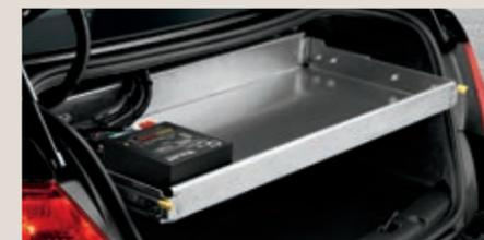
**Trunk electronics tray (Sedan only).** Aluminum, retractable locking tray installed at plant; no height adjustment.
