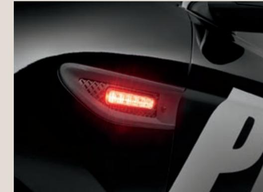
**Police side lamps.** Fender side markers feature backlit flashing, linear high-intensity LED lamps.
