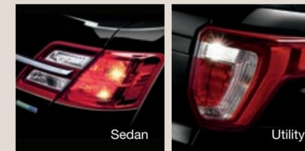
**Police taillamp.** Includes halogen base lamp, plus (2) integrated hemispheric lighthouse LED side warning lights (Sedan with red lens; Utility with white lens).
