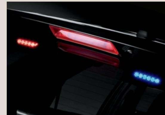
**Police liftgate-glass lights.** Includes (2) backlit flashing, linear high-intensity LED lights with surround cover (driver side red; passenger side blue) – mounted inside the liftgate glass.
