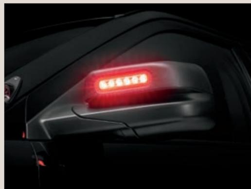
**Sideview mirror side marker LED lamps.** Features backlit flashing, linear high-intensity LED lamps.
