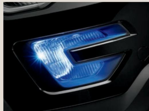
**Front warning auxiliary lamps.** Features integrated, custom-designed LED assemblies.
