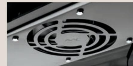
**Trunk circulation fan (Sedan only).** Wired to ignition to turn on; circulates air from the cabin to the trunk.
