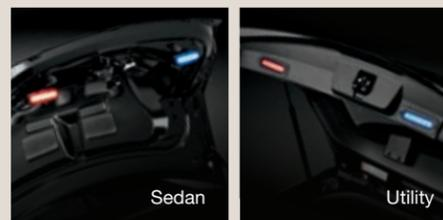
**Police rear lighting.** Includes (2) backlit flashing, linear high-intensity LED lights (driver side red; passenger side blue) – Sedan lights are mounted on the inside of the trunk decklid and Utility lights are installed on the inside lip of the liftgate. (Lights activate when trunk/liftgate is open.)
