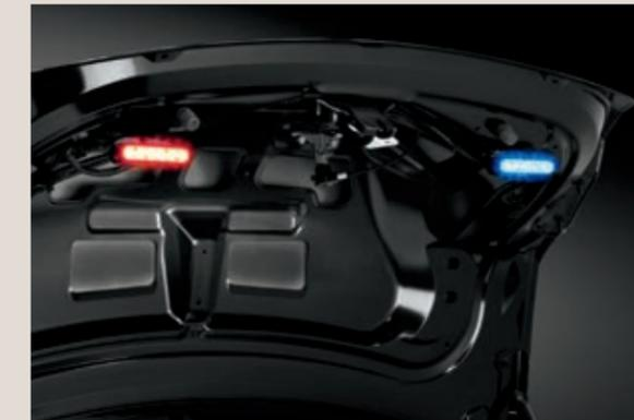
**Police trunk lights.** Includes (2) backlit flashing, linear high-intensity LED lights (driver side red; passenger side blue) – mounted on the inside of the trunk decklid. Lights activate when trunk is open.
