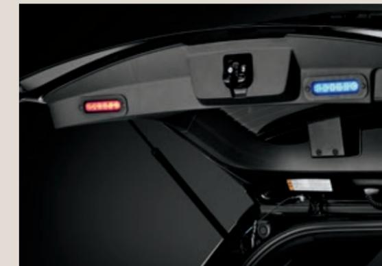
**Police liftgate lights.** Features (2) backlit flashing, linear high-intensity LED lights (driver side red; passenger side blue) – mounted inside the liftgate lip. Lights activate when liftgate is open.
