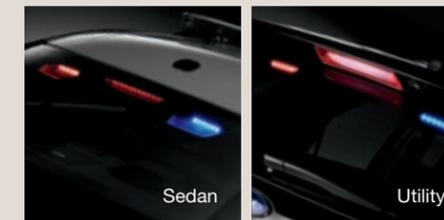
**Police rear lighting.** Includes (2) backlit flashing, linear high-intensity LED lights with surround cover (driver side red; passenger side blue). Sedan lights are mounted on the inside of the back window and Utility lights are mounted on the inside of the liftgate glass.
