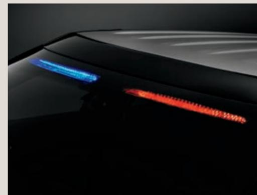
**Front interior visor light bar.** Includes (2) backlit flashing, linear high-intensity LED lights (driver side red; passenger side blue) – mounted inside the windshield glass. Lights can be programmed for tricolor (red, white, blue) patterns.
