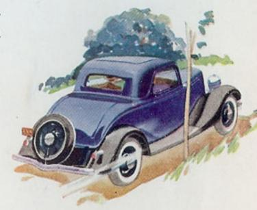
be opened outward for ventilation. A large cowl ventilator is also provided. Transverse cantilever springs give remarkable riding comfort and safety. They are attached to the axles at their flexible ends so that road shocks are taken at the most sensitive points first—and immediately controlled by four Houdaille hydraulic shock absorbers of the double action type automatically and thermostatically controlled.
