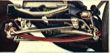
Mercury's double-action hydraulic shock absorbers are of improved design—slow-motion springs are longer than ever—for increased riding comfort. Mercury's new transverse stabilizer and anti-sway har improve car equilibrium—minimize side-sway—provide better steering control,
