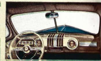
Finished in handsome grain, plastic and bright metal, Mercury's instrument panel combines unusual beauty with convenient grouping of dials and controls. Features include edge-lighted clock, glove compartment and two ash trays.
