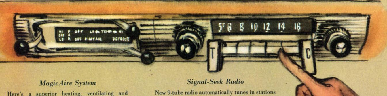
New 9-tube radio automatically tunes in stations in either direction of the dial. Town button (T) tunes local stations, Country button (C) gives broad coverage. 6-tube radio also available.
