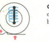
**OLD:** Conventional front springs cushion out up-down shock of bumps, but not head-on shock of bumps.
