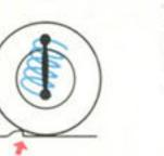
NEW: Springs tilted back allow front wheels to absorb head-on as well as up-down shocks.
