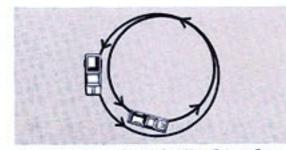
EASY TO GET AROUND IN! The Falcon Ranchero and Sedan Delivery have a compact 109.5-inch wheelbase and short overall length of 189 inches. This provides a short turning diameter and good maneuverability.
