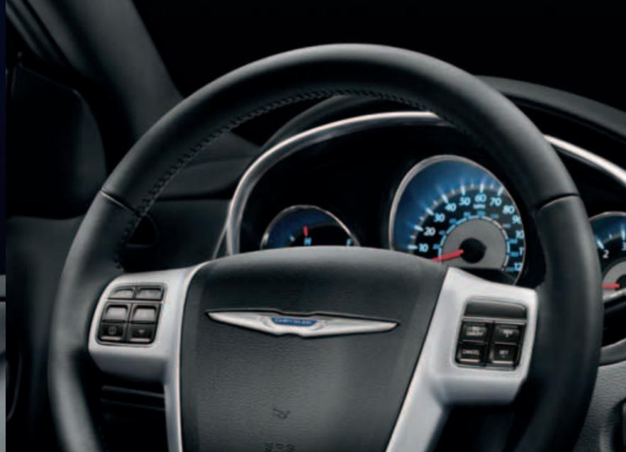
TILT/TELESCOPING STEERING COLUMN WITH INTEGRATED CONTROLS IS STANDARD
