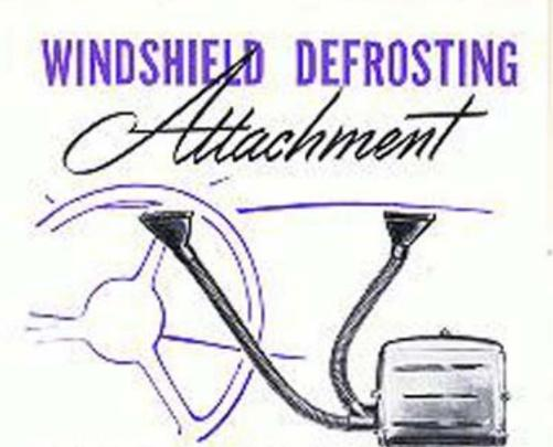
Conducts warm air from the heater to the windshield. Removes mist, frost, ice. Provides clear vision for safer driving. Operates with Super, Tri, Canadian type Tri, Deluxe and Duo Airstream Custom Built heaters.
