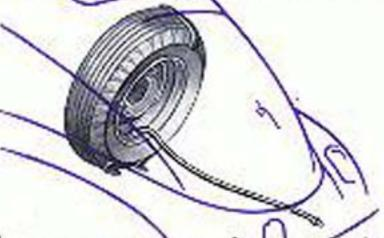
Helps assure owner of properly inflated spare—Makes it easy to check spare when checking other thes. Consists of hose and fittings for extending valve through rear apron. Eliminates unlocking and raising of rear deck lid.
