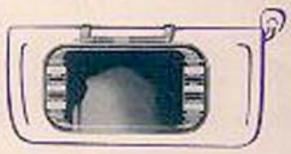
ing or leaving car. Quality mirror glass with metal shield over back. Pencil in holder for recording service and travel data in etched spaces.
