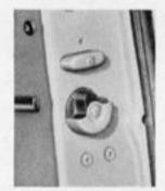
Plymouth doors can be closed quietly and opened easily. They're equipped with rotarytype door latches.
