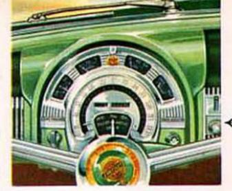
The oil and gasoline gauges; the temperature and voltage indicators; and the speedometer dial are all grouped in the Safety-Eye Instrument Cluster where they can be seen at a glance. A switch controls bright or dim lighting of the instrument panel.
