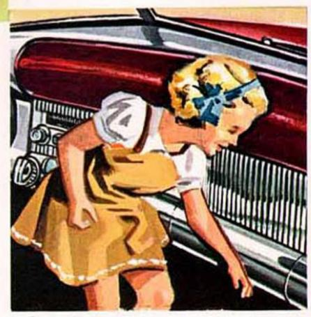
A great Chrysler safety feature for the front seat passenger . . . the Safety Crash Pad, which is made of thick sponge rubber and extends across the top of the dash panel.
