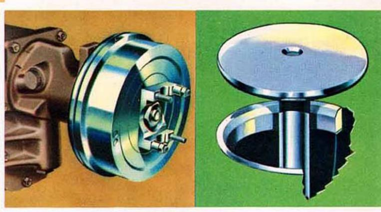
One of the great safety features on all Chrysler cars is the Safety Rim Wheel, which holds the tire on the rim in case of  $\rightarrow$  a blowout, enabling you to bring the car to a safe stop.
