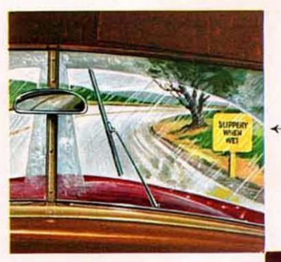
With the Chrysler Electric Windshield Wipers there is no "stop and go" action that blurs your vision. They are constant, operating at a regular speed because they are run by electricity and not by the engine. The blades have a wide sweep. There are two speeds, high and low—both constant speeds.
