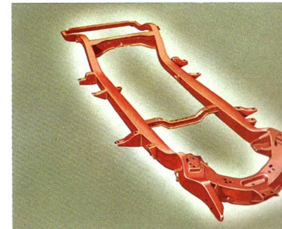
The Chrysler box-section type frame has long been known for its strength and rigidity. But, for 1955, there is a completely redesigned frame, which is, in our opinion, the finest frame ever developed for a motor car. Clean, straight lines are used throughout,
