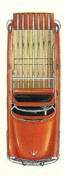
Tailgate lowers flush with floor for easy loading and unloading. Storage space is 46 in. wide; 30% in. high and 90% in. long . . . 121% in. long with tailgate down, rear seat folded forward.
