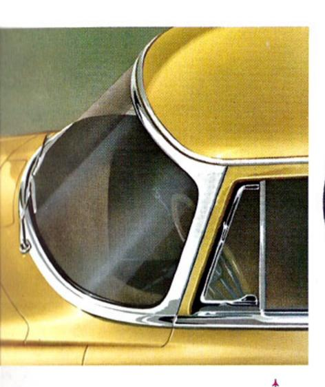
One of the outstanding design features is the "New Horizon" super-scenic windshield with the swept back corner posts that eliminate blind spots. The graceful curve and correct slanting of the windshield not only provide maximum visibility, with no distortion, but also enhance the beauty of the front end design of the car.
