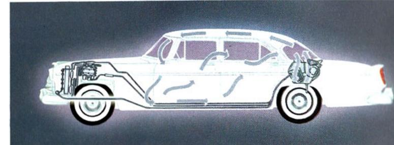
New Independent Parking Brake, working direct on driveshaft, has handle conveniently mounted on dash. Red flasher signal above lever warns driver when brake is set.
