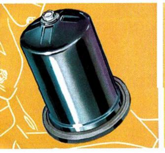
Exclusive Full-flow Oil Filter, developed by Chrysler, eliminates
