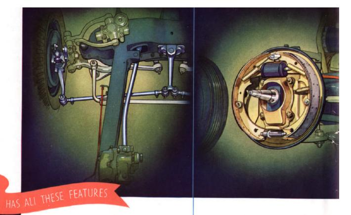
EVERY BUICK HAS BUILT-IN COIL SPRING KNEE-ACTION—and this, together with skilful weight distribution, the torque tube drive, front end ride stabilizer and air cushioned tires, accounts for the wonderfully smooth and joltless ride of the phenomenal 1936 Buicks.
