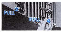
Pull out two Ventilation knobs (2) and (4)—with the right one only halfway out.
