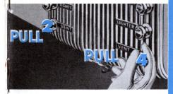
Pull out both Ventilator knobs at bottom (2) and (4).
