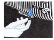
First see that the Thermostat Control (3) is all the way to right—in OFF position.
