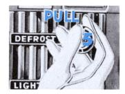
To cool air at shoulder-level, or to keep windshield and windows from fogging in wet weather, pull out Defroster knob (5).
