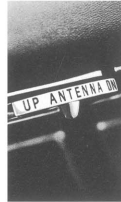
Electric Power Antenna (Code 381). Available with all radios on all models except Firebirds. Raises and lowers antenna by a switch on the instrument panel. Antenna is mounted on the right rear fender. (F, D)
