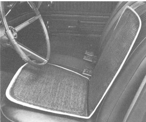
Ventilated Cushions. Helps make driving more comfortable, especially in hot, sticky weather. Special, coil-spring construction allows air to circulate between passenger and seat. (D)
