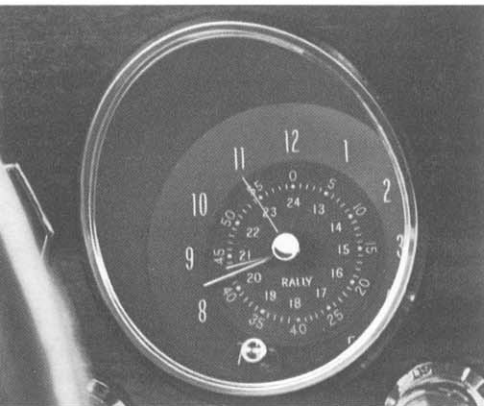
Rally Clock (Code 474). Available on Tempest, Tempest Custom, Le Mans and GTO models only—except those equipped with Code 444, Rally Gauge Cluster. Features sweep second hand and automatic self-regulator. (F, D)
