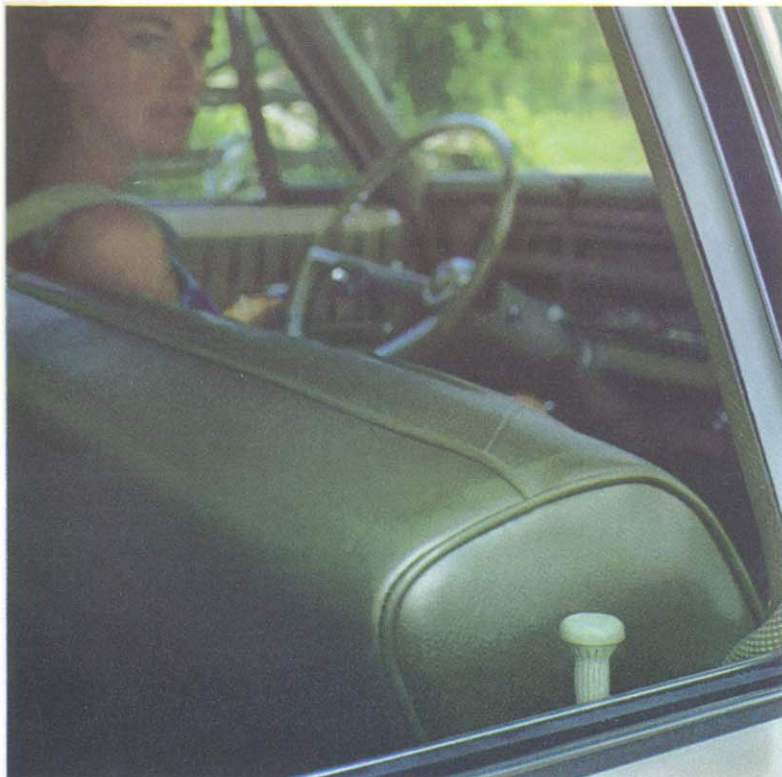
Power Window Lifts (Code 551). Gives driver fingertip control of all vertical side windows from a single control panel on his door. Each window has its individual control switch, too. Not operable with ignition key off. Standard with Brougham Option. Available on all models. (F)
