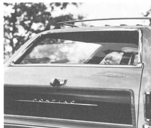
Power-operated Tailgate Window (Code 542). Conveniently located switch raises or lowers tailgate window at touch of finger or twist of key in tailgate lock. Available for Catalina and Executive 2-seat, Tempest Custom and Tempest Safari Station Wagon models only. (Standard on all 3-seat station wagons) (F)
