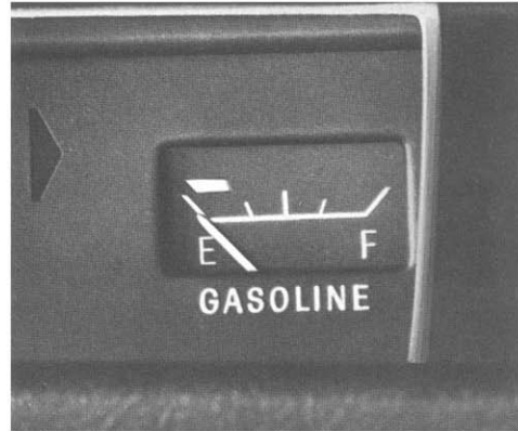
Low-fuel Warning Lamp (Code 672). Available only on Catalina, Executive, Bonneville and Grand Prix (part of Lamp Group—Code 332—for these models). Red warning light in fuel gauge alerts driver to low fuel supply. (F)
