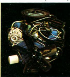
Carburetor: Semi-hemispherical combustion chamber design and dished pistons. Two barrel carburetor with large throat diameter for good fuel-air distribution. High - energy ignition system for hotter spark, eliminates distributor points and condenser. New catalytic converter emission control, located in the exhaust system. Ex-
