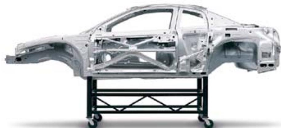
**Steel spaceframe construction.** Every three-door coupe is built on a strong, welded steel skeleton. Front and rear crumple zones are designed to help absorb energy instead of transmitting it all to the passengers. The doors are built with steel beams and cross bracing for side-impact protection. As if the intended safety benefits weren't enough, this construction also helps reduce the number of squeaks and rattles that can develop over time.
