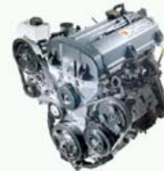
**1.9-liter engines.** The SC2 engine has a dual-overhead-cam design, has four valves per cylinder and produces 124 horsepower at 5,600 rpm and 122 ft. lbs. of torque at 4,800 rpm. The SC1 has a single-overhead-cam design, has two valves per cylinder and delivers 100 horsepower at 5,000 rpm and 114 ft. lbs. of torque at 2,400 rpm. Both engines operate on 87-octane gasoline, both have durable steel timing chains and both are available with a five-speed manual or four-speed automatic transmission.
