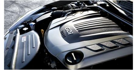
**AN INJECTION OF POWER** With every rev of its 348-horsepower GDI V6, fuel is injected directly into the cylinder, creating potent-yet-efficient combustion. Genesis Coupe's powerful stopping performance is aided by available 4-piston Brembo® brakes.
