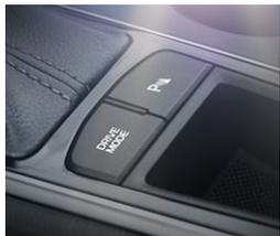
**DRIVE MODE SELECT** The 2015 Sonata comes standard with Drive Mode Select. It alters steering calibration and engine mapping to create distinctive characteristics for each of the three selectable driving modes: ECO for fuel efficiency, NORMAL for balanced performance and SPORT for dynamic steering feel and aggressive engine response.
