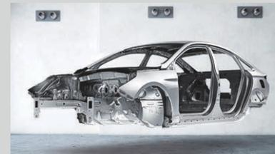
**HIGH-STRENGTH STEEL** To enhance handling precision and overall driving dynamics, the majority of Sonata's body is built with advanced high-strength steel. It's a material twice as rigid as ordinary steel, yet 10 percent lighter. It's also a big reason why Sonata performs so well for occupant protection in safety tests.
