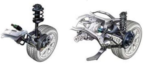
Aluminum wheels Large 18-inch wheels and tires, standard on the B9 Tribeca, help increase handling limits and can provide greater stopping power. The aluminumalloy construction reduces weight for more precise and controlled wheel movement.
