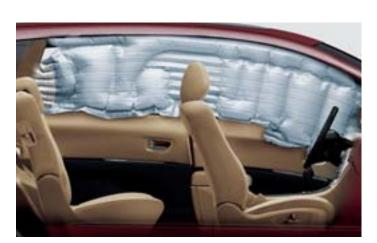
Front, side and curtain air bags An intelligent front air bag system senses driver's seat position and front-passenger seat occupancy to determine the safest deployment level for each. Front side-impact air bags are mounted to the seat to stay in position as the seat is adjusted. And side-curtain air bags help protect front and outboard 2nd-row passengers.
