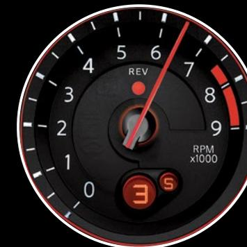
**A world's first.** Included in the Sport Package, SynchroRev Match<sup>®</sup> technology – the first in any production car – monitors the 6-speed manual's clutch pedal, shift lever and vehicle speed. As you shift to a lower gear, the system will “blip” the throttle to the ideal engine rpm for a supremely smooth downshift as you let out the clutch. The system also works when upshifting to give you a smooth flow of power when accelerating.
