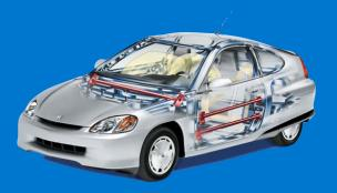
**Surround yourself.** The Insight is a bulwark of protection, thanks to Honda-developed **G-Force Control Technology** (G-CON). Each part of the body and frame-and even the wheels, suspension and spare tire-help to absorb impact energy.
