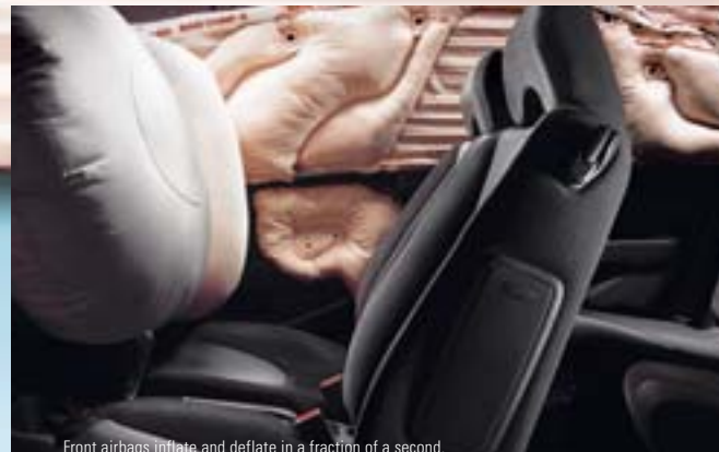
Front airbags inflate and deflate in a fraction of a second.
