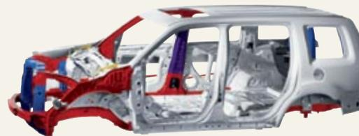
**Advanced Compatibility Engineering™ (ACE™)** body structure helps improve crash-compatibility in frontal impacts with vehicles of differing bumper heights and in offset-frontal impacts. The increased use of high-tensile steel improves the integrity of the passenger compartment.
