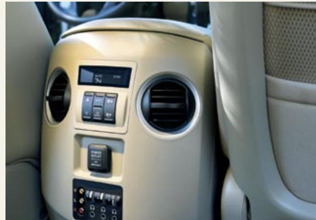
**Second row** features climate controls and a 12-volt power outlet. RES-equipped models include RCA inputs for a game console or other video source.
