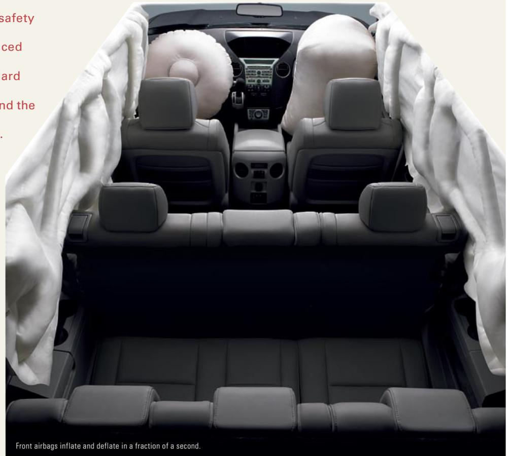
Front airbags inflate and deflate in a fraction of a second.
