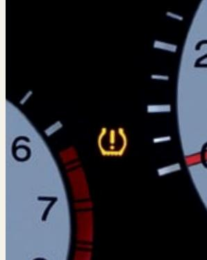
**Tire Pressure Monitoring System™ (TPMS)** notifies you with a warning indicator in the information display if air pressure in a specific tire is significantly low. Touring model gives you an individual pressure readout for each tire.
