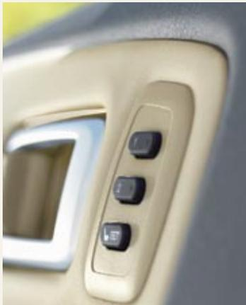
**Two-position memory** on Touring adjusts driver's seat and outside mirrors.
