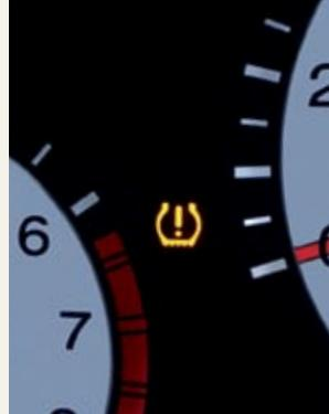
**Tire Pressure Monitoring System™ (TPMS)** notifies you with a warning indicator in the information display if air pressure in a specific tire is significantly low. Touring model gives you an individual pressure readout for each tire.
