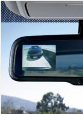
**Rearview camera** on EX-L models utilizes a portion of the rearview mirror as a full-color camera display when you engage reverse. On Touring models, the image is displayed on the vehicle's navigation screen.
