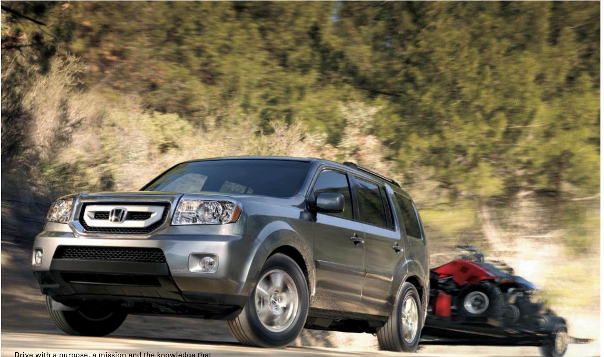
Drive with a purpose, a mission and the knowledge that you've got power to spare. The 3.5-liter i-VTEC® V-6 generates 250 hp and 253 lb-ft of torque—enough to tow up to 4,500 lbs.<sup>7</sup> Standard equipment like an integrated Class III trailer hitch, heavy-duty radiator and fluid coolers means the Pilot comes fitted with most of what you need for some serious hauling.
