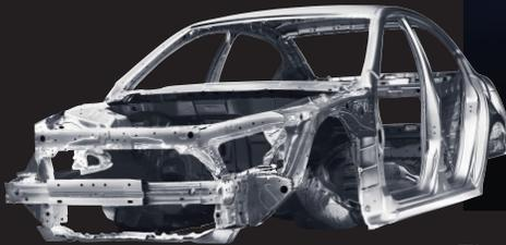
The Accord's Advanced Compatibility Engineering™ (ACE™) body structure is a Honda-exclusive body design that enhances occupant protection and crash compatibility in frontal collisions.
