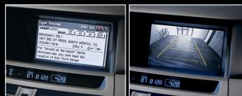
On navigation-equipped Sedan models, shift into reverse, and the rearview camera with an innovative guideline display makes it easier for you to maneuver the vehicle when backing up.
