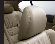
To help reduce the likelihood of whiplash injuries in a rear-end impact, the front seats have active head restraints. They move up and forward in a rear collision to help keep head movement to a minimum.
