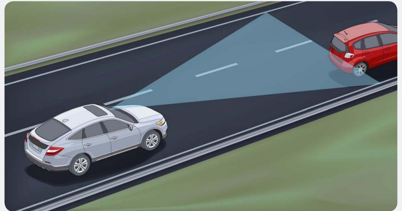
The Forward Collision Warning (FCW)<sup>7</sup> system can sense the presence of vehicles in front of you and issues alerts if it calculates that you are at risk of a collision (EX-L models).
