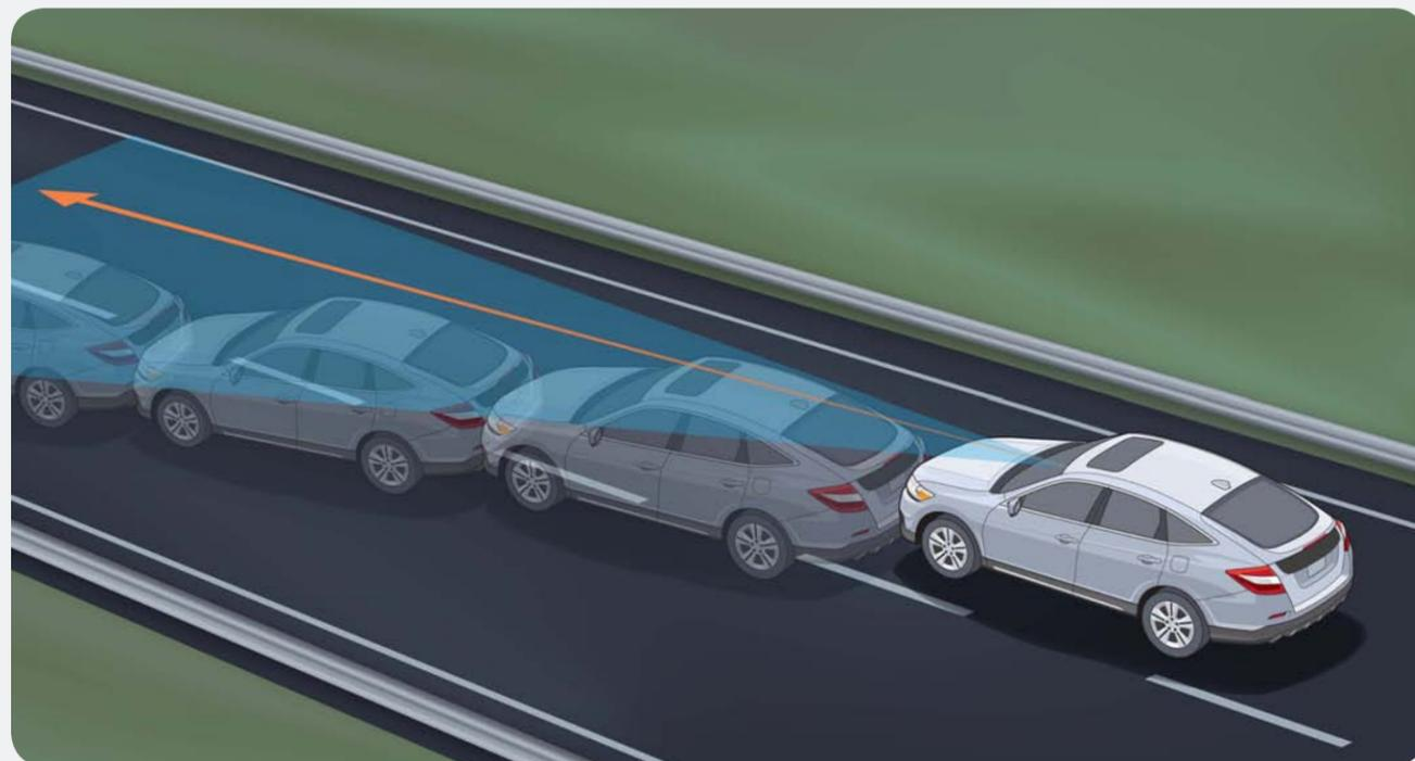
With the Lane Departure Warning (LDW)<sup>8</sup> system, a small camera between the windshield and the rearview mirror can track lane markings on the road. The system alerts you when it detects you moving into a different lane without signaling (EX-L models).
