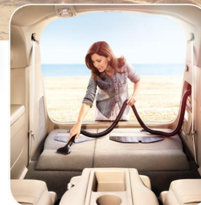
Because dirt knows no boundaries, the Odyssey's exclusive HondaVAC® goes where you need it. The vacuum is located in the driver's-side rear of the vehicle, but can reach all the way to the front-passenger area. The HondaVAC also includes two handy attachments, as well as a removable waste bin for quick and easy cleaning. (Touring Elite)
