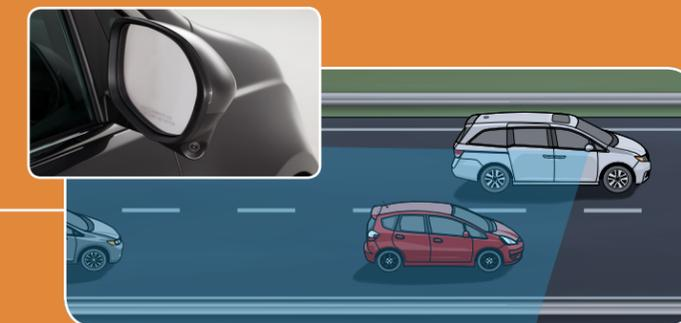
**Honda LaneWatch<sup>15</sup>** This innovative feature uses a small camera under the passenger-side mirror to greatly reduce your blind spot. When you signal right, live video displays on your i-MID screen revealing nearly four times more area than the mirror alone. (EX, EX-L, Touring)
