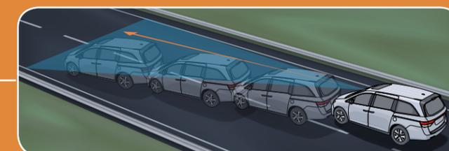
**Lane Departure Warning (LDW)<sup>16</sup>** Using a small camera behind the rearview mirror, LDW can track lane markings on the road and alert you when it detects you drifting into a different lane without signaling. (EX-L and above)
