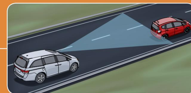
**Forward Collision Warning (FCW)<sup>13</sup>** The new FCW system can detect the presence of vehicles in front of you and issues alerts when it calculates you are at risk of a collision. (EX-L and above)
