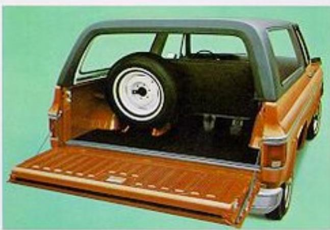
The Jimmy is as wide as a standard pickup and the effective load length behind the drivers seat is 76.6 inches. With the roof off there's room for extra bulky objects, and the load length can be extended by dropping the tailgate which is supported by strap-type steel links.
