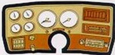
Wrap-around cockpit instrument and control cluster design places all gauges, warning lights and major controls directly in front of the driver. A gauge package is available which includes: oil pressure gauge, ammeter and coolant temperature gauge; a tachometer or clock is available with the gauge package. Foam instrument panel pad is standard.
