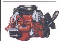
New 305 V8. Our new 305-cubic-inch engine with a 2-barrel carburetor is standard on V8 models, except in California where the 350-4 V8 is required. It has fewer cubic inches than the V8 it replaces, yet the 305 shares all the big-engine features that contribute to good performance and efficient operation: a short stroke to reduce friction, valve-in-head design for free breathing, precision-balanced crankshaft, full-jacket cylinder cooling.
