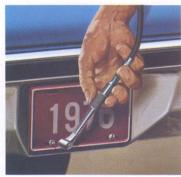
Air-adjustable shock absorbers. Standard on El Camino, air-adjustable rear shock absorbers trim the vehicle at any rated load and help prevent "bottoming out" with heavy loads. You simply stop at the nearest service station and pump air into the rear shocks through a special valve at the rear license plate.
