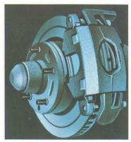
Front disc brakes: standard. These brakes are the single-piston floating-caliper type. They resist fade and recover quickly from the effects of water immersion. El Camino's rear drum brakes are finned for efficient cooling. Vacuum power assist is included.
