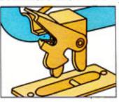
When the latches are released, as shown, the seat can be slid off the rear anchors, then lifted and removed.
