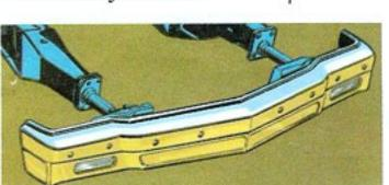
Standard bumper system uses reinforced outer bars and two hydraulic/pneumatic cylinders to cushion minor impacts.
