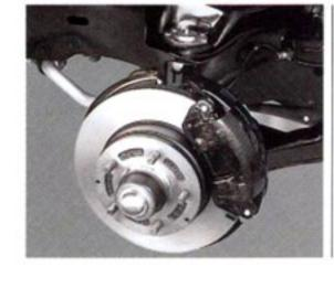
Disc Brakes Standard, Four-wheel anti-lock brakes reduce wheel lockup during severe braking and are designed to help you maintain steering control, even in a panic stop in rain or snow.
