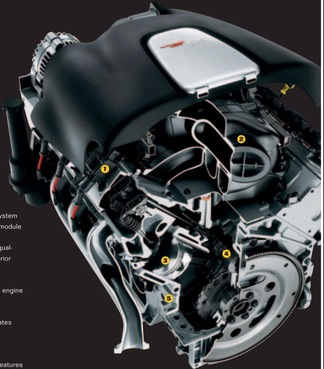
The 6.0L LS2 V8 delivers more than 300 lb.-ft. of torque from 1200 to 6500 rpm with peak torque of 400 lb.-ft. at 4000 rpm (shown with GM Accessories engine cover insert).
