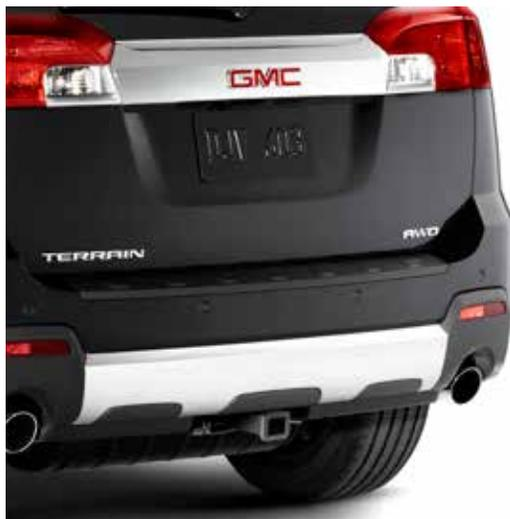
**HITCH TRAILERING PACKAGE** This structural welded steel hitch features a standard 1.25" receiver to fit most ball-mount assemblies and includes a wiring harness.
