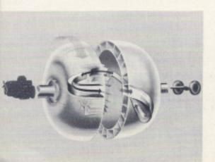
Inside the pump vane, the speed of the oil deflected by the stator is added to the speed built up by the pump. So the oil in the pump is traveling much faster than before.
