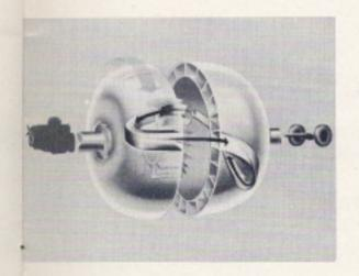
The speed and force of the oil moving through the pump is increased still more —
