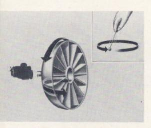
When the pump rotates, it pumps oil by centrifugal force—the same force which causes a weight twirled on a string to fly outward. Oil is thrown from the inner ends of the vanes outward, and it gushes from the outer ends.
