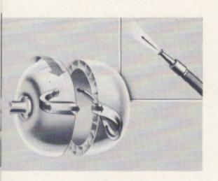
However, when the oil leaves the turbine it has a lot of energy left. And each turbine vane acts like a hose nozzle because the vane is smaller at the inner end.
