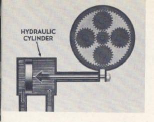
Bands are applied and released by oil from hydraulic cylinders, controlled by the pilot control lever.
