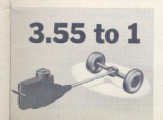
The third member is the Econo-MISER High-Reduction Rear Axle. Rear axle ratio has been decreased from 4.11 to 3.55 to one — to take fullest advantage of the power in the new engine, and to assure economical driving.
