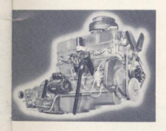
Now, let's examine briefly the second and third members of Chevrolet's Automatic Power Team. First, there's the great new 105 Horsepower Valve-in-Head Engine — the engine specifically designed for the POWERGLIDE Automatic Transmission.
