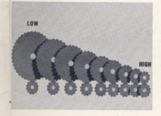
The ideal transmission would have an infinite number of gear ratios arranged in tiny graduations to provide just the right amount of power for every step in acceleration. This is impractical with gears.
