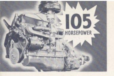
Equally as important as the automatic transmission, the new engine is a combination of new design and time-proved features. It is, of course, valve-in-head design—and such advantages as complete, uniform cooling, specialized four-way oiling and castiron pistons have been retained.
