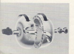
And when the turbine approaches the speed of the pump—equivalent to high gear—there is not enough oil circulation through the vanes to cause further power multiplication.
