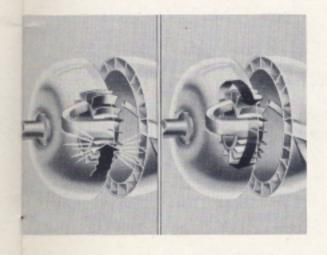
So the stator is mounted so that when pushed from one direction it will not move—while pressure from the other direction causes it to turn freely.
