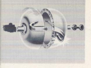
Because of the shape of the turbine vanes, the oil also pushes on the turbine—to take more advantage of the twisting action. But there is still no power multiplication.
