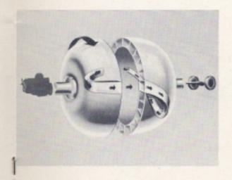
When the engine is idling, the pump turns slowly and the motion of the oil does not move the turbine.
