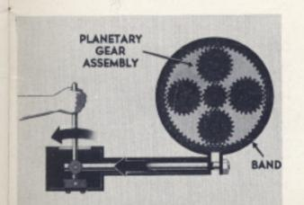
The emergency low and the reverse gears are called "planetary" gears. The ratio—or direction of rotation—is changed by clamping the outer gear with a band, without the gears actually shifting.
