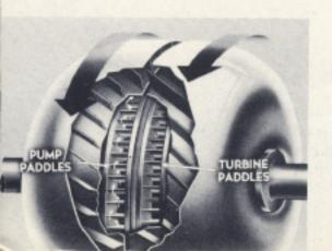
This is done by paddles in the pump and turbine, arranged so that when the pump is turning faster than the turbine, its paddles slide through the oil with little effect.
