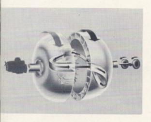
As the turbine picks up speed, the oil flow through the vanes slows down. So there is less and less power multiplication.
