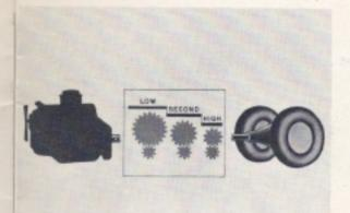
Gear transmissions usually contain only three speeds forward. So exactly the right amount of power multiplication is obtained at but three points in acceleration, with a power interruption at each shift.
