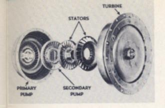
This is what the transmission looks like. Actually there is the pump, a secondary pump, two stators, and the turbine. And there are some other refinements.
