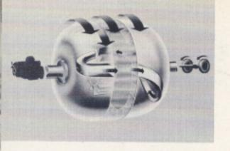
Then, as the turbine picks up speed, oil pressure begins to come from the other direction and the stator begins to turn.
