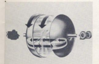
However, the fluid coupling alone cannot multiply power. On a grade, or with a heavy load, the pump simply spins—and the turbine cannot move.
