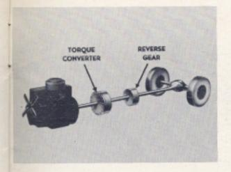
We have seen that no gears are used in the POWERGLIDE Automatic Transmission. But, since the oil flow cannot be reserved, a reverse gear is required.
