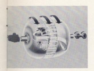
However, the stator, which directs the oil in the right direction to help multiply power, would interfere with the oil if it remained stationary as the transmission approaches the high driving range.
