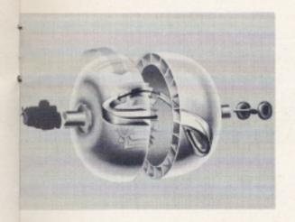
So the oil, moving still faster, is again deflected into the pump.
