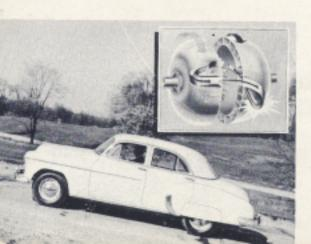
Of course, if the car starts up a grade—or if you accelerate at low speeds—so that the turbine is turning more slowly than the pump, circulation through the vanes again increases and you have exactly the amount of power multiplication needed.
