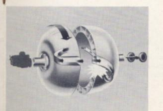
Then, when the engine is speeded up, the pump throws more oil into the turbine, where it exerts its twisting power.
