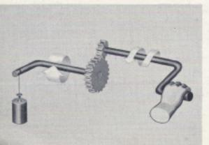
A gear with a certain amount of twisting power on its shaft can produce twice as much on the shaft of a gear twice as large. Naturally, the larger gear turns only half as fast.
