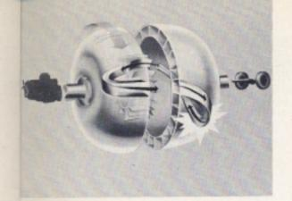
And when the oil re-enters the turbine, it exerts more force. Power has been multiplied because the oil is traveling with more force than the pump alone could provide. However, it still may not move the turbine.
