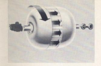
The oil is also surging from pump to turbine, and a way was found to move it in this direction with more force than the pump alone could impart.
