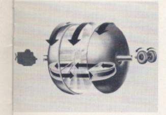
Meanwhile, the oil returns from the turbine—through the pump—back through the turbine—around and around. The oil is transferring engine power to the rear wheels.
