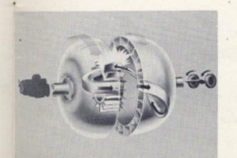
Thus, when power multiplication is needed, the force of the oil from the turbine vanes holds the stator rigid.
