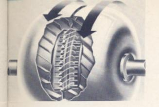
However, when the turbine turns faster—as on a downgrade or when the accelerator is released—the turbine paddles throw oil against the pump paddles. This tends to couple the units and provide engine braking.
