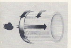
Because of the shape of the vanes, the oil gets away from the pump. The flow from all the vanes forms a rotating, cylindrical jet of oil, moving away from the pump.
