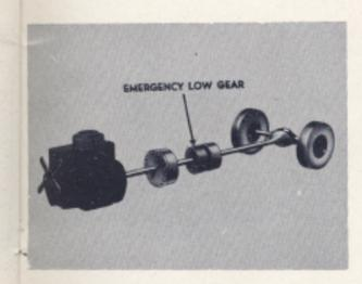
And to assure ample power for every emergency, a low gear is added. The automatic transmission alone can multiply power by more than two times, and the low gear multiplies it again by nearly as much — giving a combined low of 4 to 1. This is much more powerful than the usual passenger car low.
