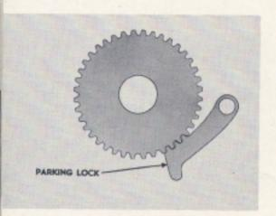
Finally, for the parking lock, a toothed lever meshes with teeth on the reverse gear drum. This drum is connected with the rear wheels, locking them when the lever is engaged.
