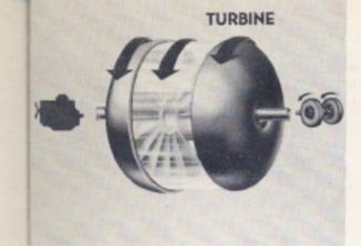
When the turbine is placed facing the pump, the oil enters the turbine vanes and twists the turbine—so the turbine turns.
