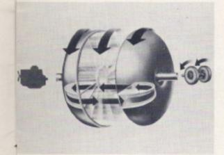
Once the turbine and the rear wheels have started to turn, they gain speed — until the turbine is turning about as fast as the pump and the rear wheels are up to driving speed, although this may take some time.
