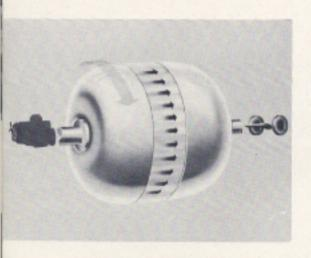
In the fluid coupling, the only means of transferring power is the surging oil from the pump. So to multiply power, a way had to be found to make the oil move faster than the pump could move it.
