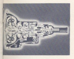
Chevrolet's new POWERGLIDE Automatic Transmission is the last word — not only in operation, but also in durability. It is manufactured and assembled with maximum precision in a new, especiallyequipped plant. And since all parts operate in oil, wear is almost nonexistent.
