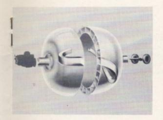
To accomplish this, the turbine vanes were reshaped to permit the easiest possible oil flow and to take fullest advantage of the oil's twisting force.
