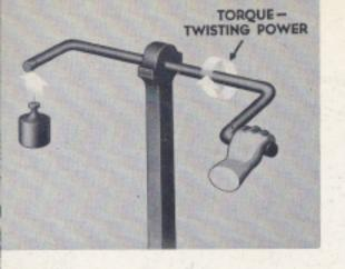
Technically, the POWERGLIDE Automatic Transmission is known as a torque converter. So we should understand that torque is simply an engineering term for measuring twisting power—and it's this kind of power we'll be referring to from now on, rather than horsepower.
