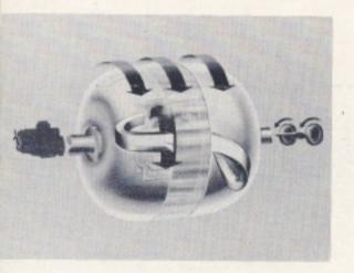
Finally, pump, stator, and turbine are all turning together —
