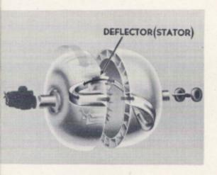
Then, a series of fixed deflectors, called a stator, directs the oil from the turbine back into the pump—in exactly the same direction as the flow of oil through the pump.
