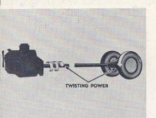
It's the twisting power of the engine which turns the wheels of the car. And it takes more twisting power to turn the wheels when starting or on a grade, than when the car is moving on the level.
