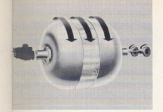
At this point the pump, all the oil, and the turbine are moving together — transferring engine power directly to the rear wheels.
