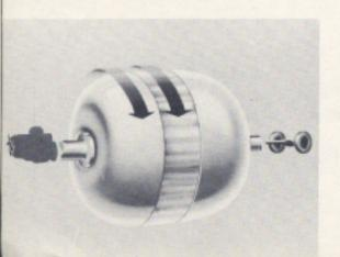
Obviously, the oil cannot rotate faster than the pump. However, the oil is not only rotating.
