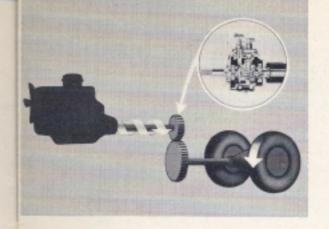
Thus, the gear transmission multiplies engine power and passes it on to the rear wheels.
