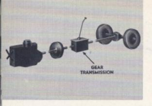
So in cars with a simple fluid coupling, a gear transmission must be used—requiring shifting, either by hand or automatically.
