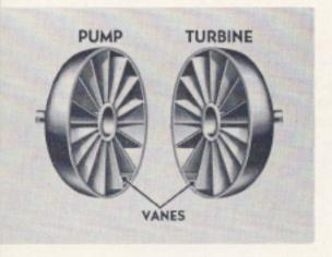
The fluid coupling has a pump driven by the engine and a turbine which drives the wheels. Both have vanes which curve outward from near the hub. When assembled, the vanes form a doughnut-shaped section, and the whole assembly is filled with oil.
