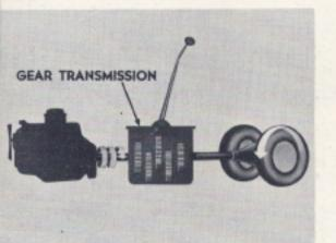
So there must be some device to multiply the engine power when necessary. A gear transmission is the traditional device used to do this. And the gear transmission principle is simple.
