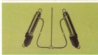
AIR-BOOSTER REAR SHOCK ABSORBERS on all El Caminos, can be inflated to provide extra load capacity.
