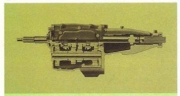
STANDARD 3-SPEED TRANSMISSION is easily operated by a shift lever on the steering column.
