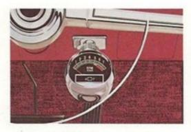
TACHOMETER—for use with either sixor eight-cylinder engines; provides an accurate check of engine revs up to 7000 rpm; helps determine exact shift points.
