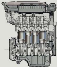
**THE 1.4L I6V MULTIAIR ENGINE** This exclusive FIAT technology, a decade in the making, utilizes electrohydraulic valves for more dynamic and direct control of air and combustion. Power is improved up to 10 percent, torque goes up 15 percent and fuel efficiency has a 10 percent advantage over conventional naturally aspirated engines. Emissions, in turn, are cut an impressive 10 percent. The MultiAir engine boasts 101 horsepower at 6,500 rpm and 98 lb-ft of torque at 4,000 rpm.
