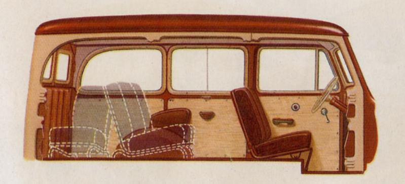
LUXURIOUS AND PRACTICAL INTERIOR with body and door panels in aspengrain finish, easy to keep clean. Armrests for driver and passengers upholstered to match simulated leather seat coverings. Both paneling and upholstery are easily cleaned by wip-
