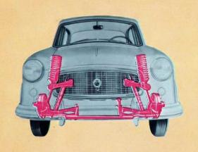
Deep Coil Front Springs, longer and softer than those used on most other cars and angled inward to control sway on curves, help make the American the smoothest riding 5-passenger car. New shock absorbers level the roughest roads.
