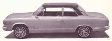
In addition to the standard Rambier American exterior trim items, the 440 has the new rally-style moldings on lower body, drip rail, rear pillar base, and rear panel. Rear panel also has "engine-turned" insert and gas cap cover. New "map-style" wheel discs are optional.
