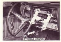
erator to the full limit which operates electrical controls to effect the shift to third. When pedal is released, the shift back to overdrive is made automatically if car speed is above 34 to 37 mph (27 to 29 for V-8).
