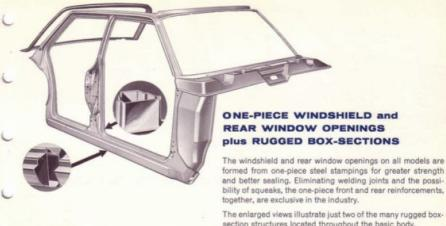
formed from one-piece steel stampings for greater strength and better sealing. Eliminating welding joints and the possibility of squeaks, the one-piece front and rear reinforcements.
