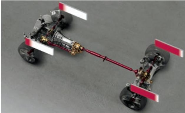
In normal driving conditions, virtually all torque is distributed to the rear wheels providing signature Jaguar rear wheel drive performance.
