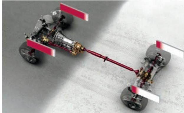
Where road conditions are changing, up to 100% of torque can be distributed to the front wheels as required to ensure optimum traction.
