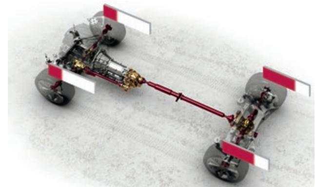
At the touch of a button Winter Mode can be selected to automatically distribute 30% of the torque to the front wheels and 70% of the torque to the rear wheels maximising control in difficult conditions.
