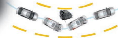
**Electronic Stability Control (ESC).** ESC helps prevent oversteer or understeer during an evasive maneuver by applying corrective forces to each of the wheels. In other words, it helps you maintain control when you need it most.
