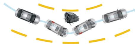
**Electronic Stability Control (ESC).** ESC helps prevent oversteer or understeer during an evasive maneuver by applying corrective forces to each of the wheels. In other words, it helps you maintain control when you need it most.
