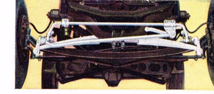
DUAL STABILIZERS mark an important improvement in the famous "Ford velvet ride." A track bar has been added to keep steering stable. The torsion bar controls sidesway.
