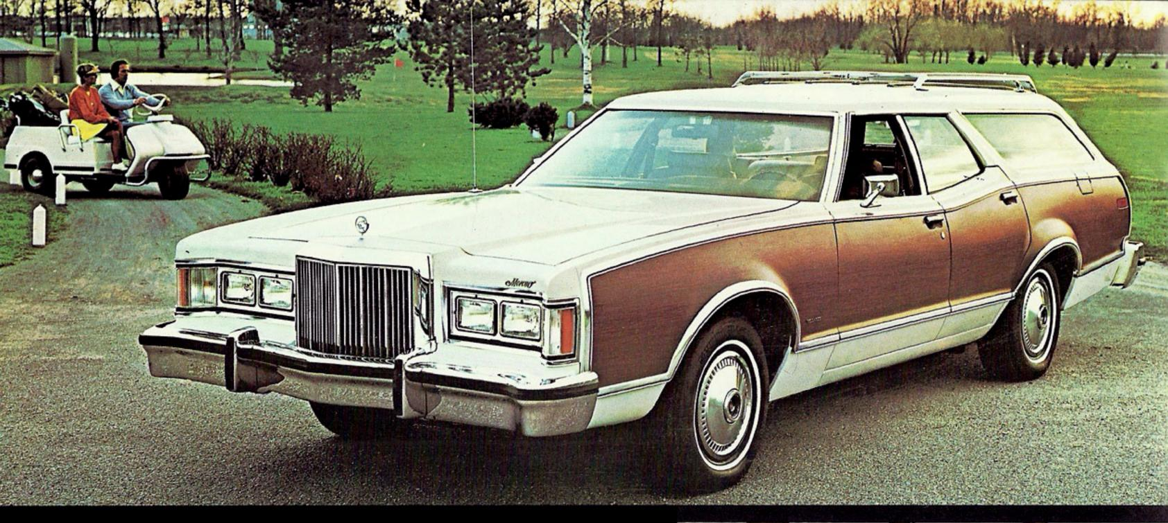
Woodgrain bodyside and tailgate treatment with bright molding and deluxe wheel covers are standard on Cougar Villager. Optional luggage rack features an integral air deflector and an adjustable bar to accommodate varying load sizes.
