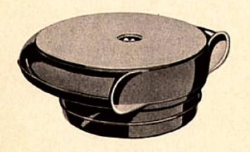
More air is needed for more horsepower! For this reason, Oldsmobile engineers designed a new air cleaner and a new intake silencer with greater capacity to accommodate the deep-breathing requirements of the new 160 horsepower "Rocket." The new air intake system also provides quieter, more efficient engine operation. What a Power Team!
