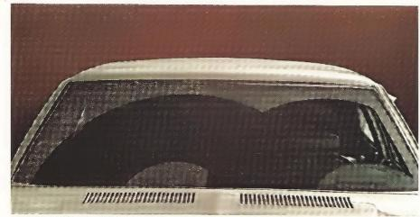
Concealed Windshield Wipers. Another Pontiac innovation. These wipers stay completely out of sight when not in use, giving a much neater appearance. And the left blade is articulated—which means it wipes clean into left corners and edges of windshield to help give the driver a wide view of the road. (Available on Tempest.)
